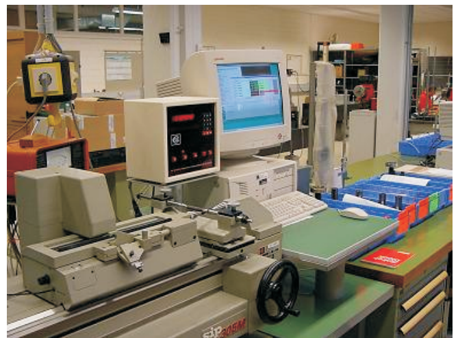
Fig. 1. Tool measuring centre at MANN+HUMMEL with EiQMI workstation
